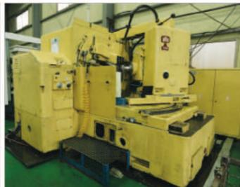
■ Straight Bevel Gear Coniflex Generator
