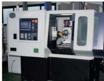
■ YH603B CNC Spiral Bevel Gear Generator
