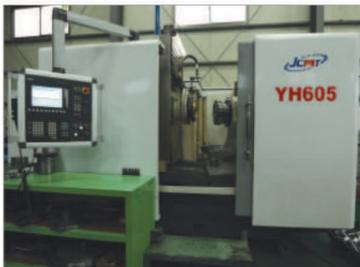
■ YH605B CNC Spiral Bevel Gear Generator
